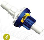
Twist the blue lock ring clockwise until the final audible "CPC Click" is heard (90° from the initial starting point). Alignment of the long blue lock ring rib indicator with the white body's rib indicator confirms initial rotation is complete.
